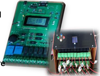
Multiplexer PV-IV Tracer System
